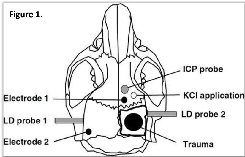
**Figure 1:** In this image, the black square represents the removal of the cranial skeleton to allow access to the trauma area, defined as the black circle. The two electrodes allow for DC measurement, which in turn amplifies the input to the EEG allowing for easily facilitated readings. The two LD probes are the locations of the probes for the measurements for intracranial pressure. The empty circle is where the KCl is injected into the brain to further depolarize and spread the CSD (6).
